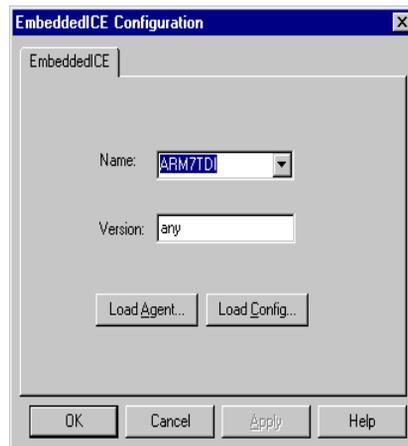
**Figure 9-20 Configuration of EmbeddedICE target**
